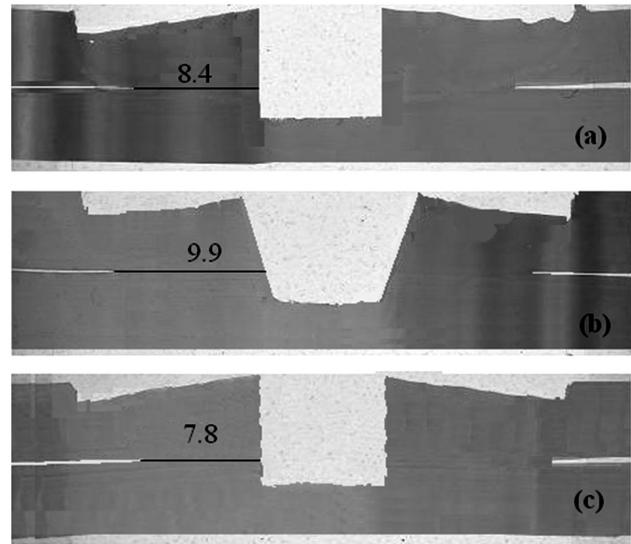
**Figure 5:** Effect of tool geometry on weld-nugget formation: a) straight cylindrical pin, b) 15° angled tapered cylindrical pin and c) threaded cylindrical pin
