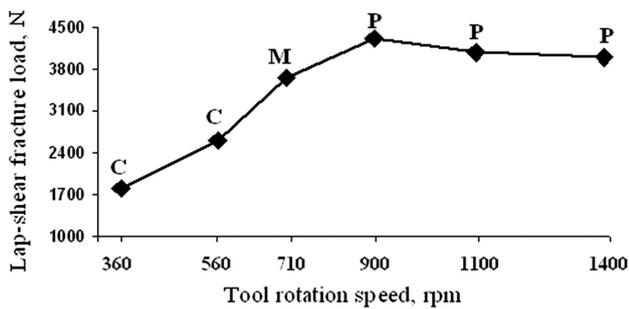
**Figure 6:** Effect of tapered cylindrical pin on lap-shear fracture load
