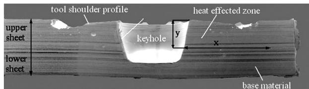
**Figure 1:** Schematic illustration of the cross-section of a friction-stir spot weld ( $x$ : nugget thickness,  $y$ : the thickness of the upper sheet and  $t$ : the total material thickness)
