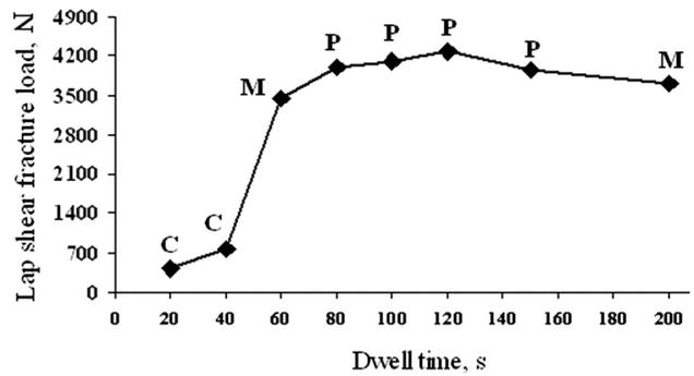
**Figure 7:** Effect of dwell time on lap-shear fracture load
