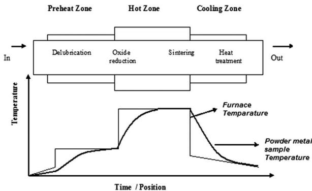
**Figure 3:** Schematic presentation of the temperature profile during medium-frequency induction-heated sintering<sup>25,40</sup>
