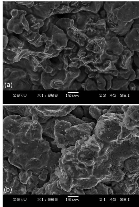
**Figure 9:** SEM microstructure of the fracture surface of an induction-sintered specimen: a) centre and b) edge of an iron-based PM compact including  $w = 3\%$  Cu ( $\times 1000$ )
