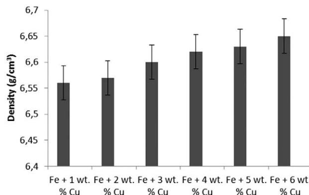
Figure 7: Density results for the PM compacts sintered with the induction system
