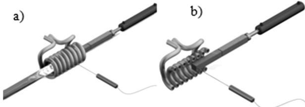
**Figure 2:** a) General aspect of the induction-sintering mechanism, b) cross-sectional aspect of a sintering action showing a sample and pyrometric temperature measurement
