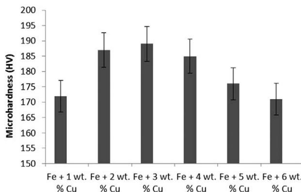
Figure 6: Microhardness results for the PM compacts sintered with the induction system
