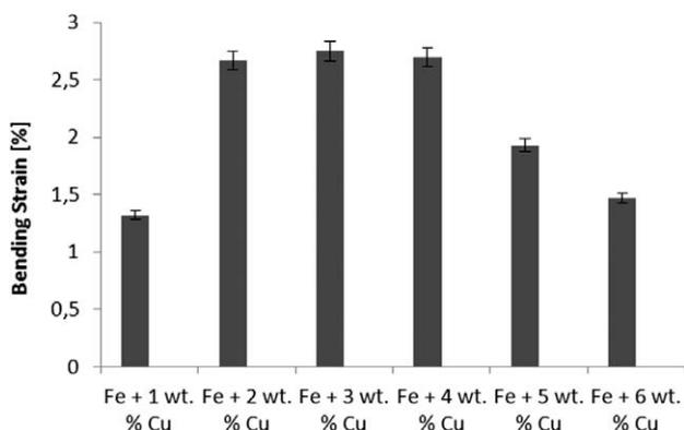
Figure 5: Bending-strain results for the PM compacts sintered with the induction system
