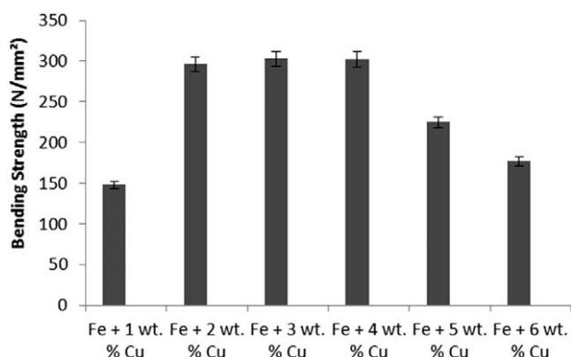
Figure 4: Bending-strength results for the PM compacts sintered with the induction system
