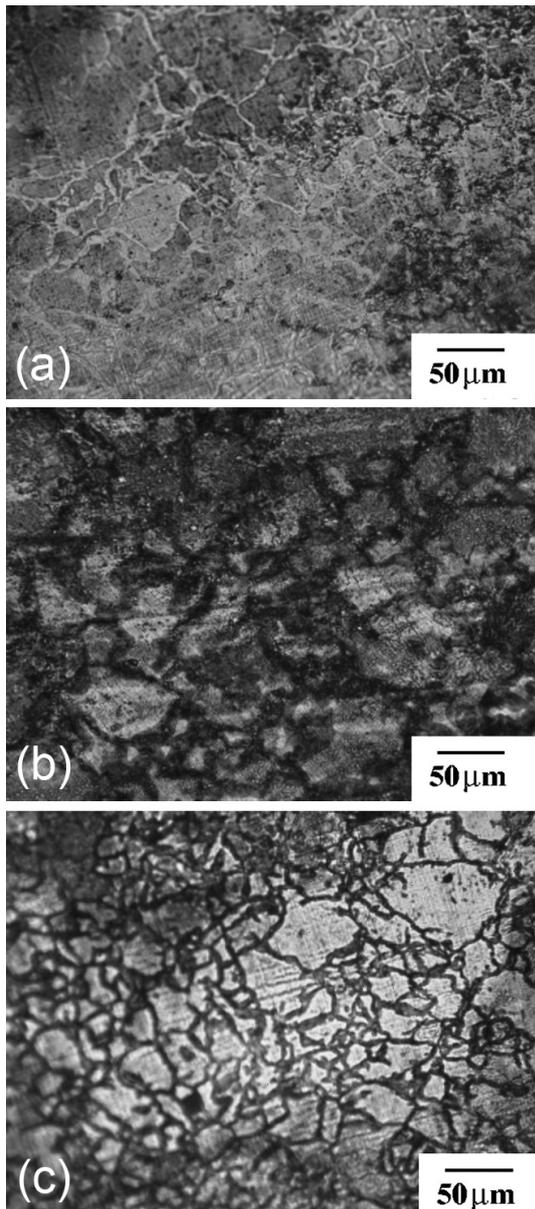
**Figure 8:** Microstructures of induction-sintered iron-based PM compacts including: a)  $w = 1\%$ , b)  $3\%$  and c)  $6\%$  Cu
