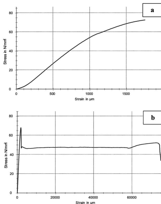
**Figure 3:** Typical  $\sigma - \varepsilon$  curves: a) for PMMA and b) for TPC
