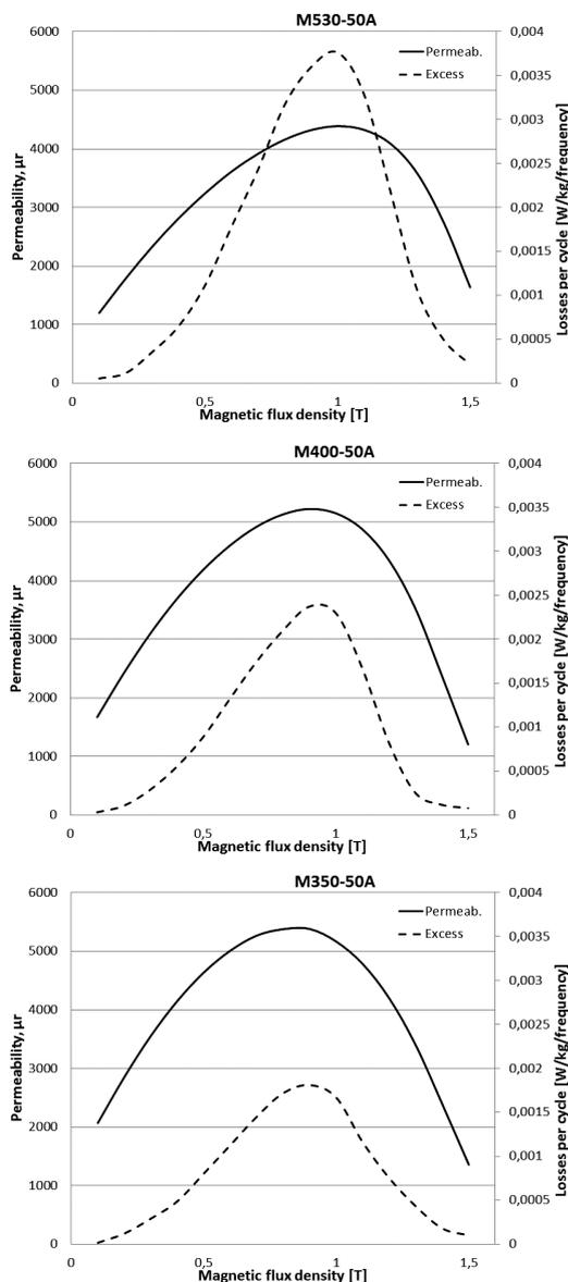
**Figure 2:** Permeability and excess losses, measured and calculated at 50 Hz in a sinusoidal waveform
