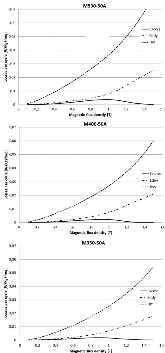
Figure 1: The aspect of the separated core losses per cycle for the investigated grades
