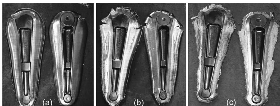
**Figure 4:** Shapes of the forgings from the magnesium alloys: a) AZ31, b) AZ61, c) AZ91
