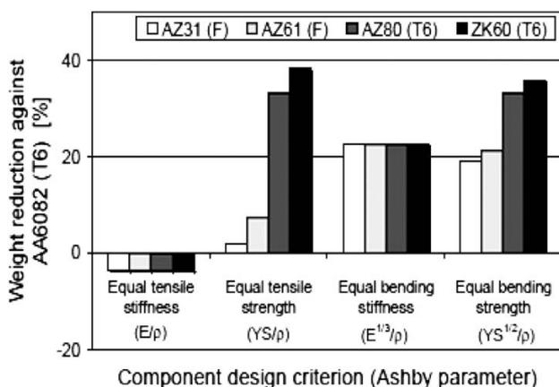
Figure 2: Mass-saving potential of magnesium over aluminium for some typical loading situations<sup>3</sup>
