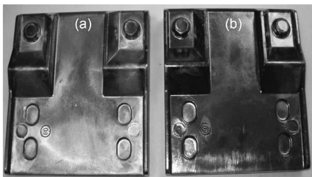
**Figure 5:** Shapes of the forgings from the magnesium alloys: a) AZ31, b) AZ61
