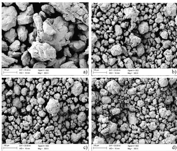
**Figure 3:** Shape and size of  $\text{Cu}_{47}\text{Ti}_{34}\text{Zr}_{11}\text{Ni}_8$  powder after: a) 7 h, b) 8 h, c) 9 h, d) 10 h of mechanical alloying, (SEM, magnifications 500-times)
