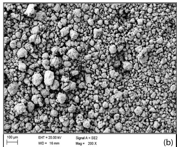
**Figure 4:** a) EDS spectrum with marked EDS X-ray lines and b) SEM micrographs of  $\text{Cu}_{47}\text{Ti}_{34}\text{Zr}_{11}\text{Ni}_8$  powders after 10 h of mechanical alloying with 30 min interruption
