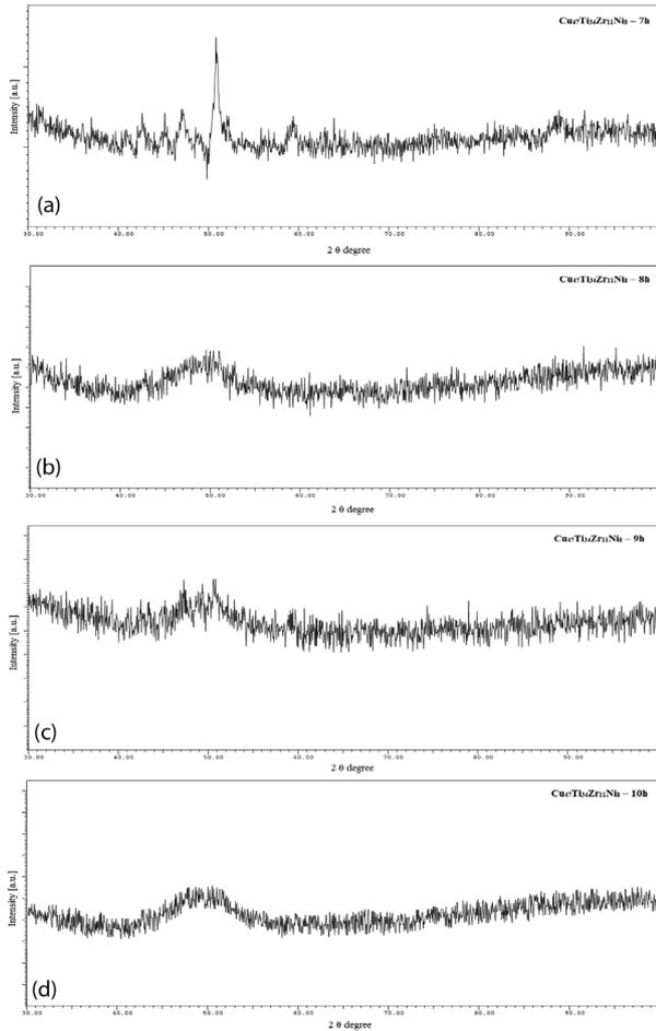
**Figure 2:** X-ray diffraction pattern of  $\text{Cu}_{47}\text{Ti}_{34}\text{Zr}_{11}\text{Ni}_8$  powders after: a) 7 h, b) 8 h, c) 9 h, d) 10 h of mechanical alloying
