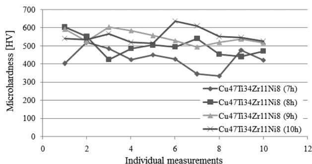
**Figure 5:** Powders microhardness after different milling times
