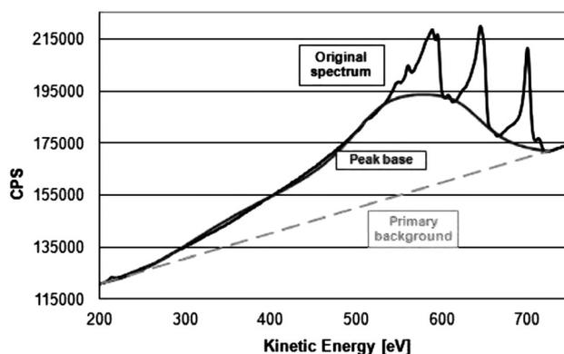
Figure 2: The AE spectra constituent elements: the primary background, the peaks base, and the peaks
