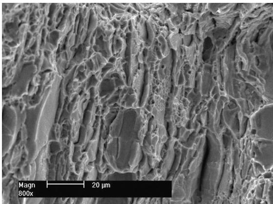
**Figure 10:** Fracture surface of the specimen aged at 700 °C for 1 h
