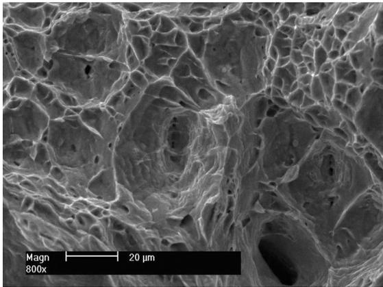
**Figure 9:** Fracture surface of the specimen aged at 500 °C for 1 h
