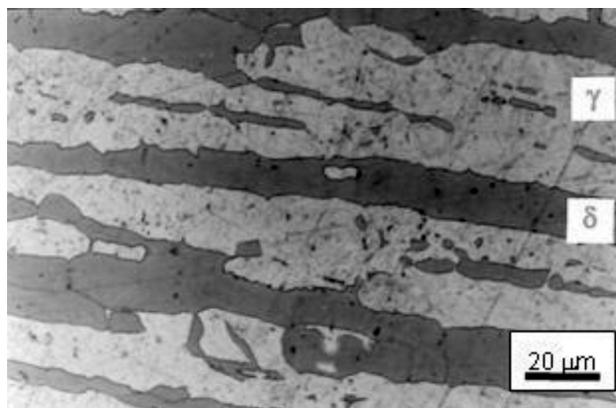
**Figure 2:** Microstructure of the as-delivered 2205 duplex stainless steel
