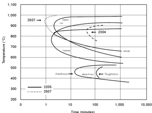
**Figure 1:** Isothermal precipitation diagram for duplex stainless steels, annealed at 1050 °C<sup>4</sup>
