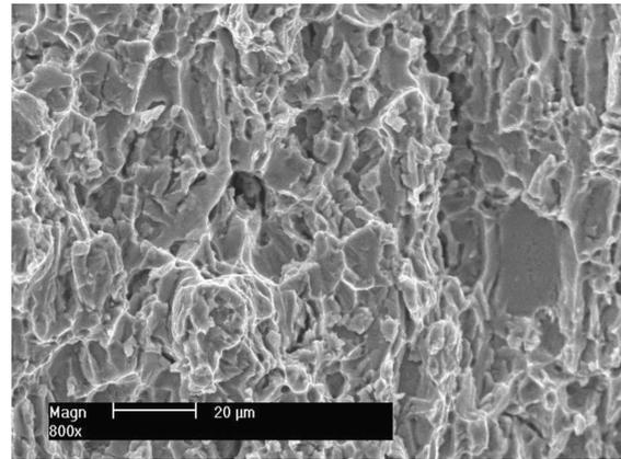
**Figure 11:** Fracture surface of the specimen aged at 900 °C for 1 h
