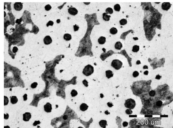
**Figure 2:** In-stream inoculation, Nital etched
