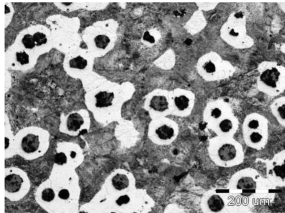
**Figure 3:** In-mold inoculation, Nital etched
