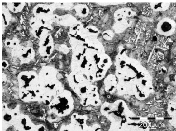
**Figure 1:** Ladle inoculation, Nital etched
