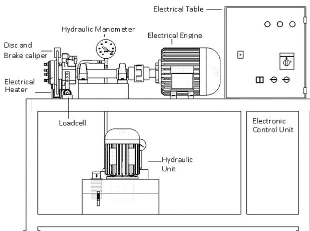
**Figure 1:** Schematic view of the brake tester
