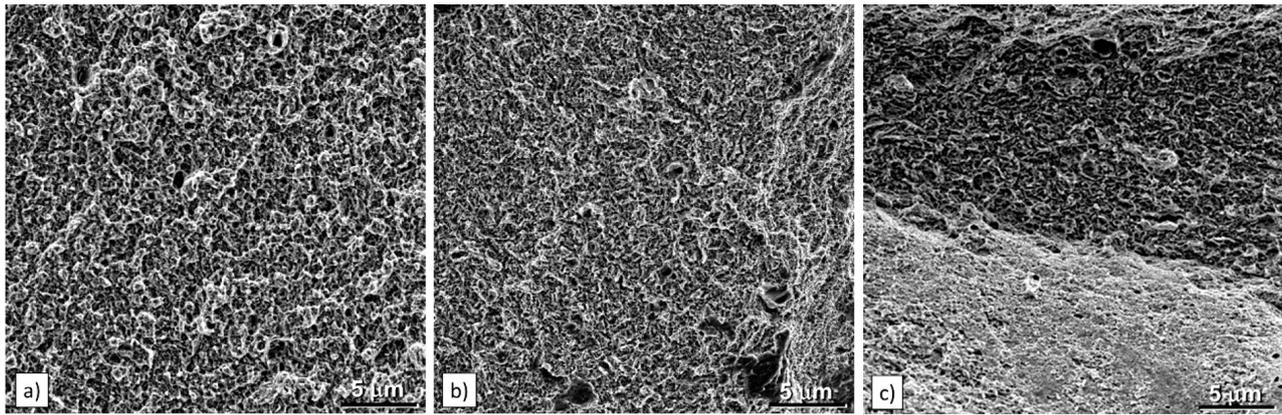
**Figure 6:** Fracture surfaces: a) T3 ( $Q_{200\text{ °C}} - C_{\text{air}}$ ) product that was cooled in air (T3/3), b) T6 ( $Q_{205\text{ °C}} - C_{\text{air}} - A_{280\text{ °C}}$ ) that was cooled in air and then annealed in a furnace (T6/3), c) T7 ( $Q_{200\text{ °C}} - P_{260\text{ °C}}$ ) product after Q&P process (T7/3)
