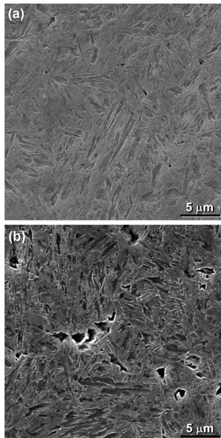
**Figure 7:** T3 ( $Q_{200\text{ °C}} - C_{\text{air}}$ ) product upon air cooling: a) martensite-bainite microstructure (point T3/2), b) martensite-bainite with a small fraction of ferrite (point T3/12)
