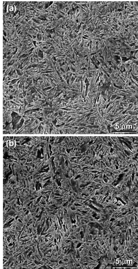
**Figure 9:** T7 ( $Q_{200}^{\circ}\text{C} - P_{260}^{\circ}\text{C}$ ) product upon Q&P process: a) martensite-bainite microstructure with a small fraction of ferrite (point T7/2), b) martensite-bainite with a small fraction of ferrite (point T7/12)
