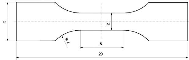
**Figure 5:** Shape of specimen for mechanical testing
