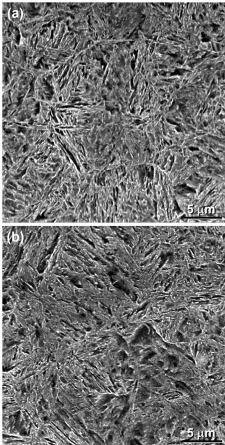
**Figure 8:** T6 ( $Q_{205}^{\circ}\text{C} - C_{\text{air}} - A_{280}^{\circ}\text{C}$ ) product upon air cooling and annealing: a) tempered martensite-bainite microstructure (point T6/2), b) tempered martensite-bainite microstructure (point T6/12)
