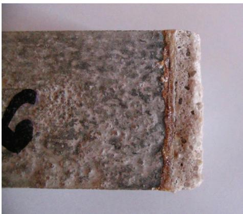
**Figure 1:** Lower part of SRP concrete sample after being in  $H_2SO_4$  0.5 % for 6 months
