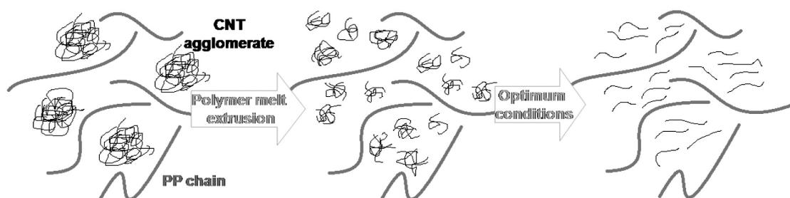
**Figure 1:** Exfoliated nanocomposite formation during the polymer-melt mixing
