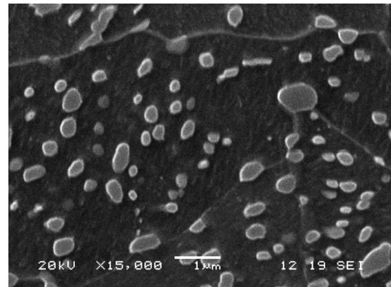
**Figure 1:** Conventionally soft-annealed sample
