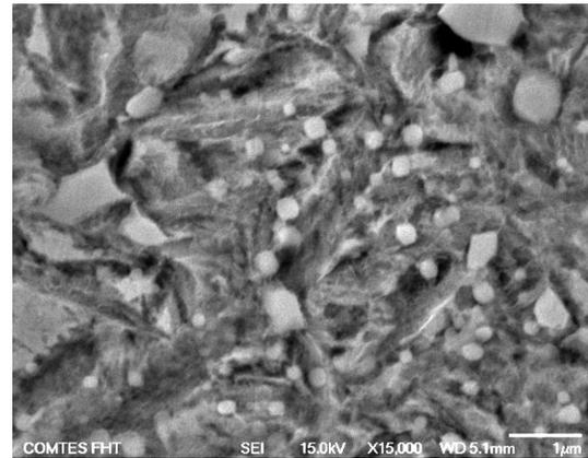
**Figure 6:** ASR-treated sample quenched from 800 °C
