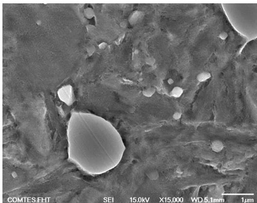
**Figure 5:** Soft-annealed sample quenched from 800 °C
