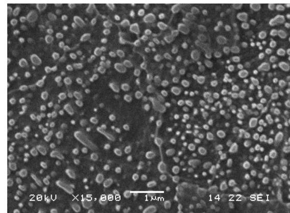
**Figure 2:** ASR-treated sample with finer carbides
