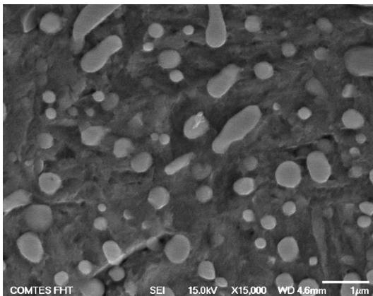
**Figure 4:** ASR-treated sample quenched from 800 °C
