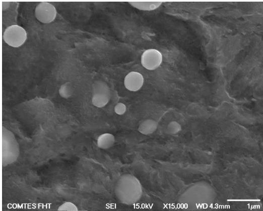
**Figure 3:** Soft-annealed sample quenched from 800 °C
