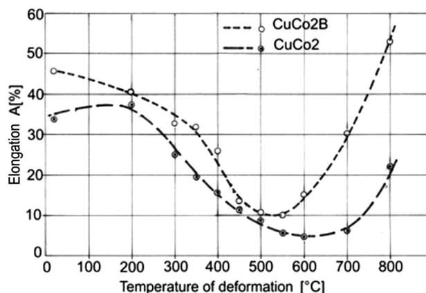
**Figure 1:** The influence of the temperature of plastic deformation in the tensile test on the elongation ( $A$ ) of the alloys CuCo2 and CuCo2B
