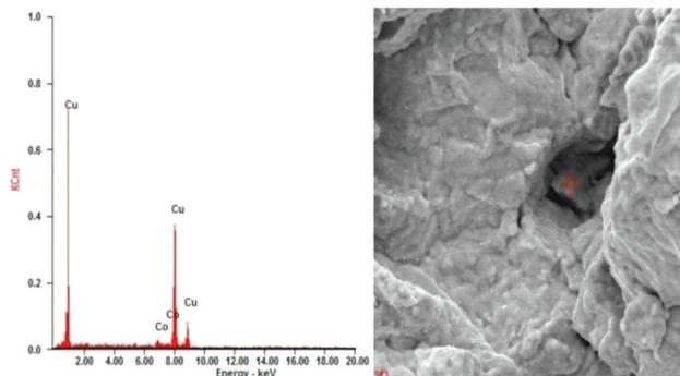
**Figure 13:** Result of the quantitative microanalysis of the chemical composition of a precipitate in the alloy CuCo2 after a tensile test at 550 °C
