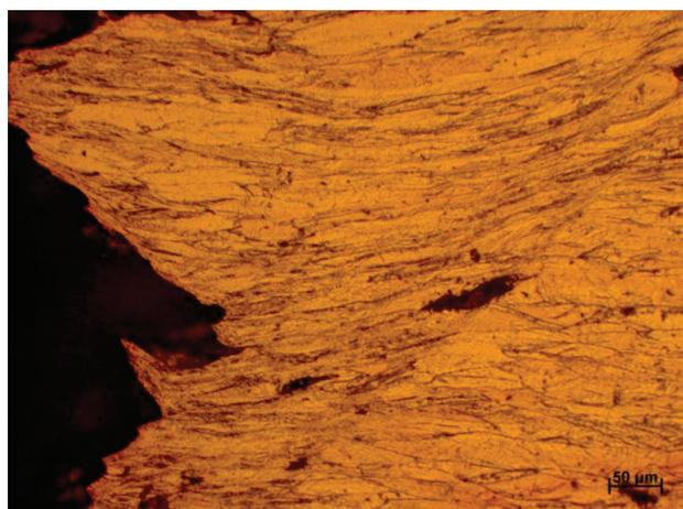
**Figure 4:** Elongated grains of the phase  $\alpha$  with a micro-crack in the structure of the alloy CuCo<sub>2</sub> after stretching at temperature of 200 °C (zone of rupture)
