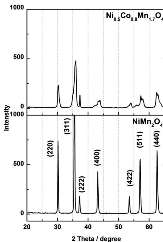
**Figure 1:** XRD patterns of  $\text{NiMn}_2\text{O}_4$  (A1) and  $\text{Ni}_{0.5}\text{Co}_{0.8}\text{Mn}_{1.7}\text{O}_4$  (A6) samples in the  $2\theta$  range 20–65°
