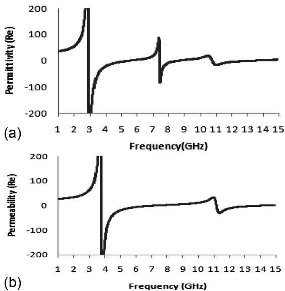
**Figure 3:** a) Real magnitude of permittivity ( $\epsilon$ ) against frequency, b) real magnitude of permeability ( $\mu$ ) versus frequency
