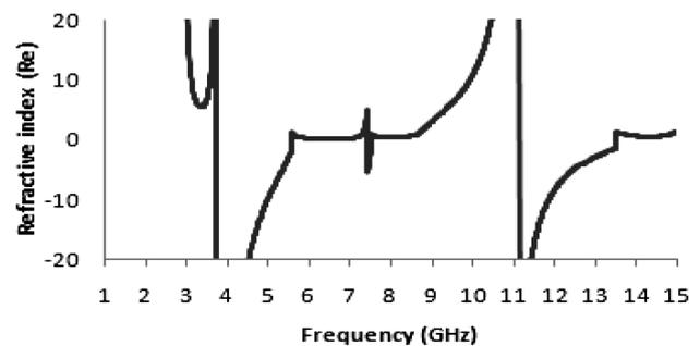
**Figure 4:** Real magnitude of refractive index ( $\eta$ ) versus frequency
