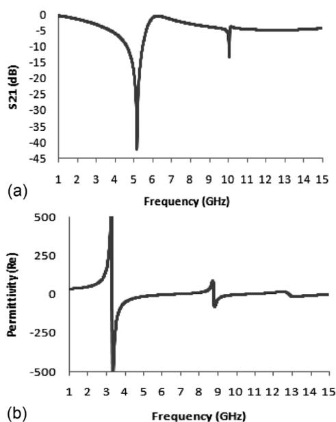
**Figure 5:** a) Transmission coefficient ( $S_{21}$ ) for the unit cell on the Rogers 6010 substrate material, b) real magnitude of permittivity ( $\epsilon$ ) against frequency for the unit cell on the Rogers 6010 substrate
