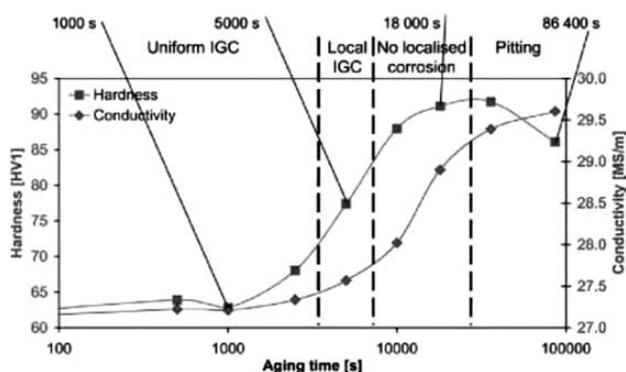
Figure 1: The dominant corrosion types in a material aged at 185 °C, according to<sup>5</sup>
