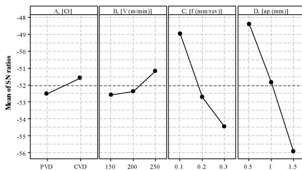
**Figure 4:** S/N graph for cutting force
