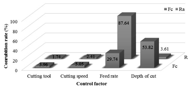
**Figure 6:** Percentage contribution of the control factors for cutting force and surface roughness
