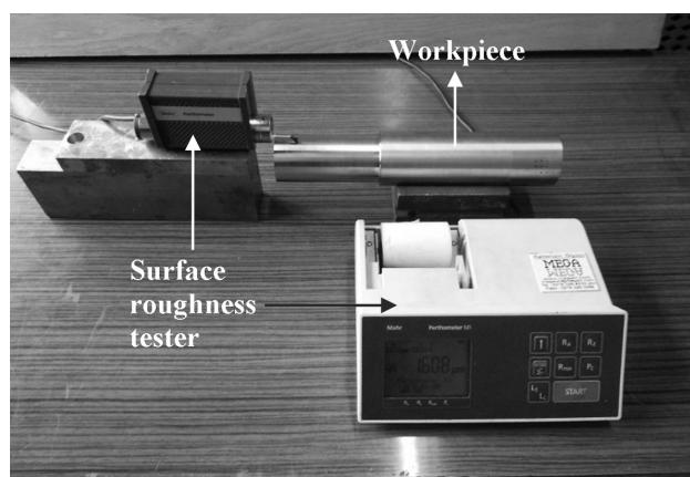
**Figure 3:** Surface-roughness measurement
