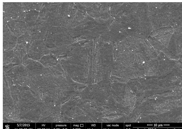
**Figure 1:** Microstructure of the precipitation-hardened 15-5 stainless steel
