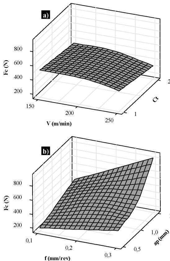
**Figure 7:** Effect of cutting parameters on cutting force: a) cutting speed and cutting tool, b) feed rate and depth of cut
