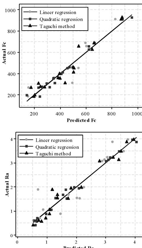
**Figure 9:** Comparisons of actual predicted values for: a) cutting force and b) surface roughness
