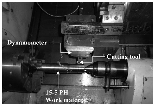
**Figure 2:** Experimental configuration for the measuring of cutting force
