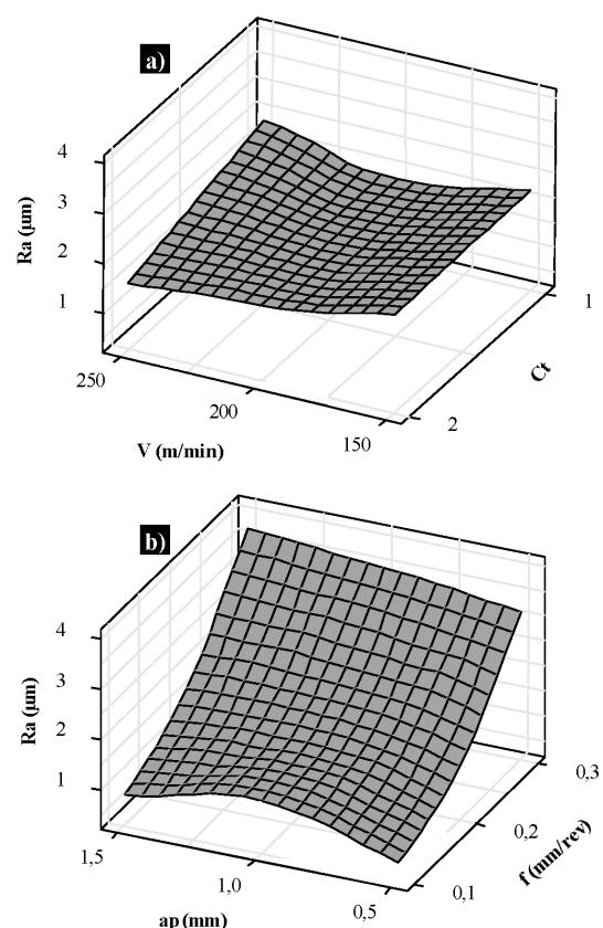
**Figure 8:** Effect of cutting parameters on surface roughness: a) cutting speed and cutting tool
