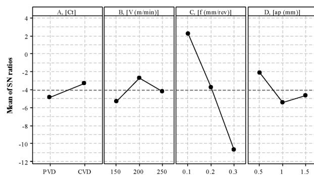
**Figure 5:** S/N graph for surface roughness
