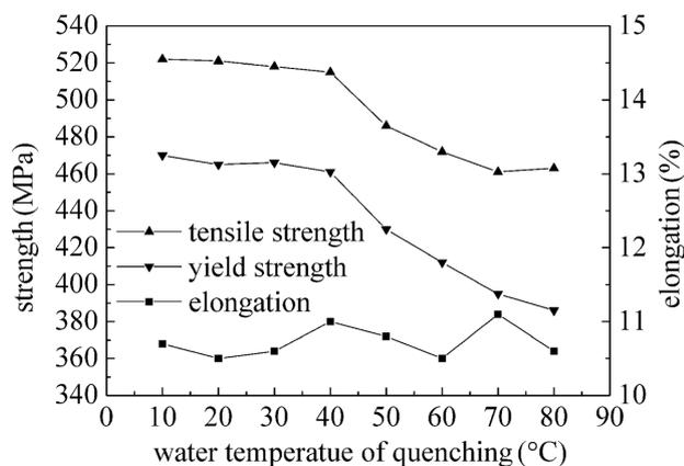
**Figure 3:** Mechanical properties changing with water temperature of quenching
