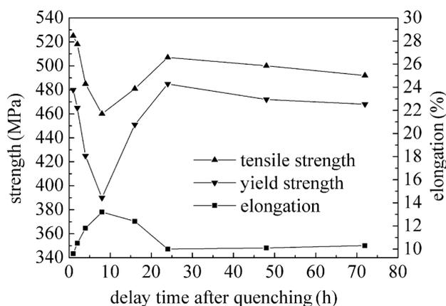
**Figure 5:** Mechanical properties changing with delay time after quenching
