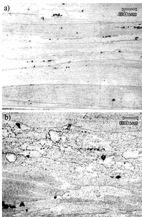
**Figure 2:** Microstructure at different solution temperatures: a) 470 °C, b) 500 °C
