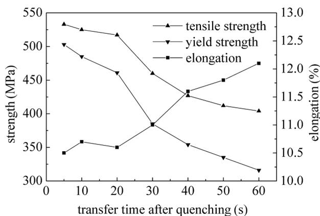
**Figure 4:** Mechanical properties changing with transfer time before quenching
