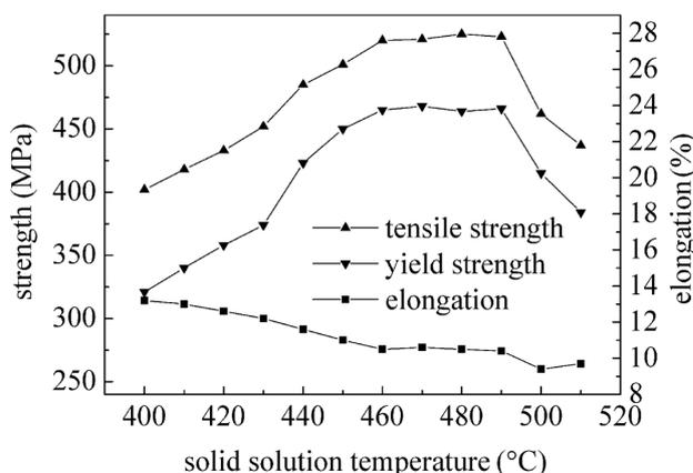
**Figure 1:** Mechanical properties changing with solution temperature
