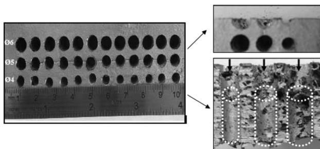
**Figure 5:** Pictures of drilling surface and holes section of Al foam sample
