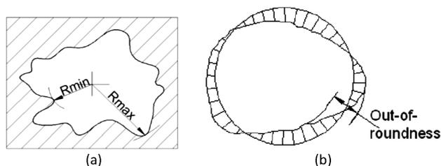
**Figure 3:** Circularity measurements: a) DFC-deviation from circularity, b) LSC-least squares circle.<sup>12</sup>
