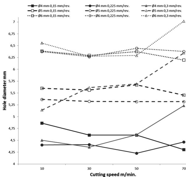
**Figure 8:** Variations in the hole diameters depending on the cutting parameters and cutting conditions
