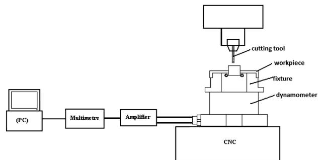
**Figure 2:** Test set-up
