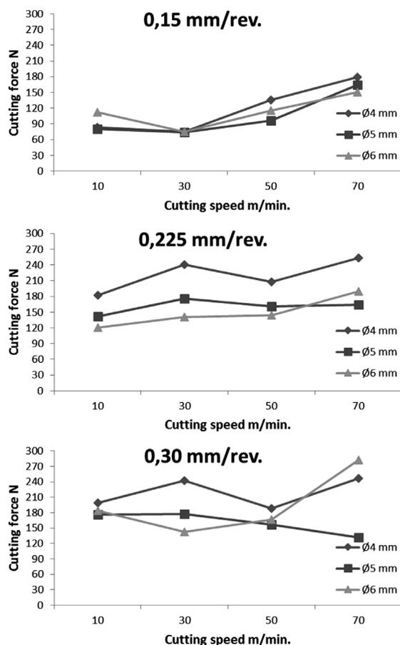
**Figure 6:** Variation in feed force depending on the cutting speeds, feed amount and drill diameter
