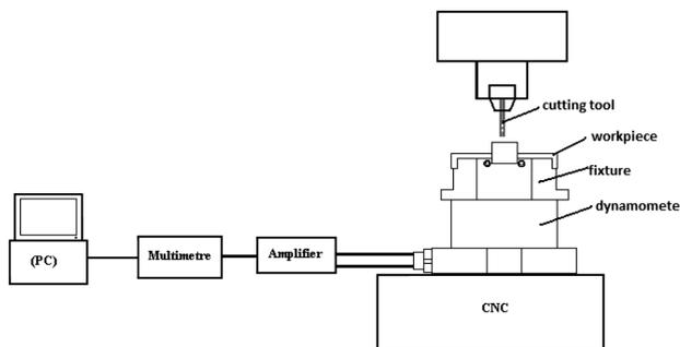
**Figure 2:** Test set-up
