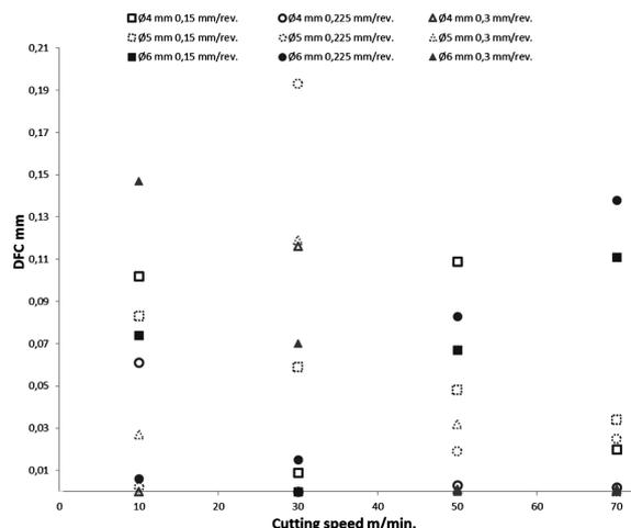
**Figure 9:** Variations of *DFC* depending on cutting parameters and cutting conditions
