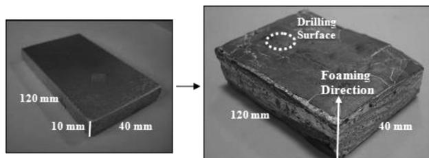
**Figure 1:** Sample picture before and after foaming process
