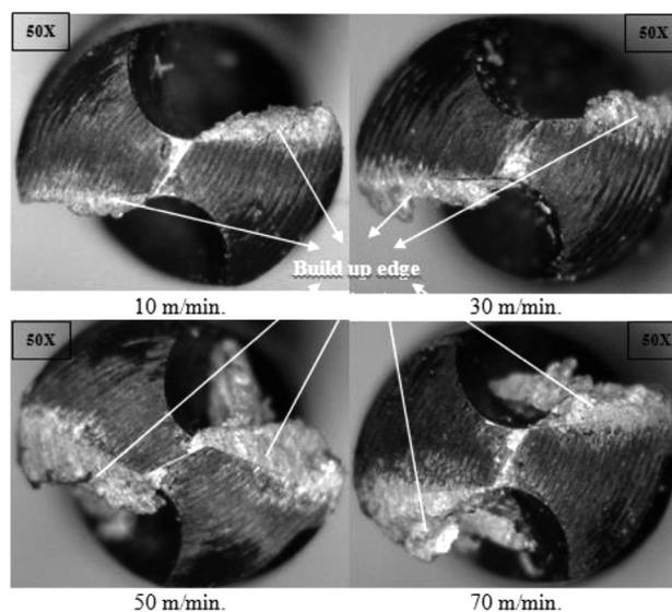
Figure 7: Built-up edge on the cutting tool with the increasing cutting speed
