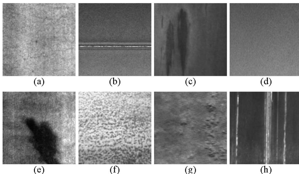
**Figure 5:** Sample images of surface defects of hot-rolled steel sheet: a) crazing, b) folding, c) inclusion, d) original, e) patch, f) pitted surface, g) rolled-in scale, h) scratch. Surface defects of steel sheet are different in direction, scale, etc.
