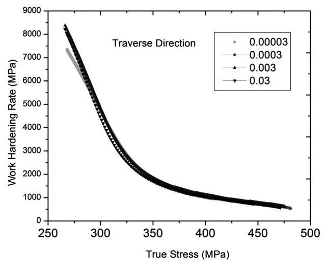
**Figure 8:** Work hardening rate – true stress relation in the traverse direction
