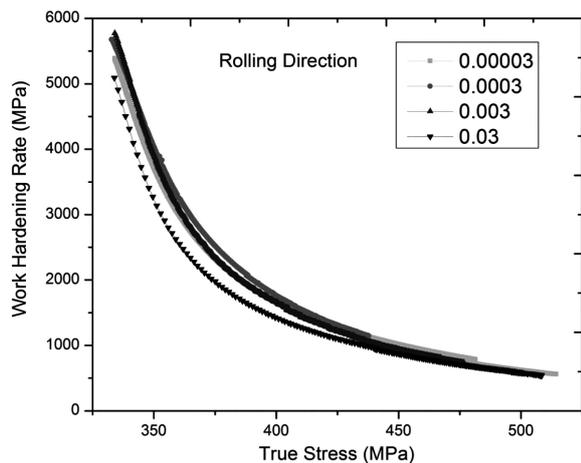
**Figure 9:** Work hardening rate – true stress relation in the rolling direction
