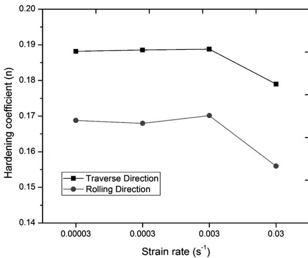
**Figure 5:** Hardening coefficient – strain rate relation
