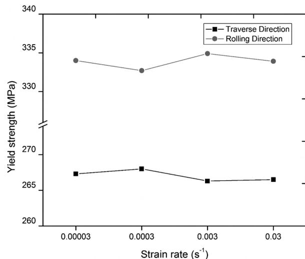
**Figure 2:** Yield strength – strain rate relation
