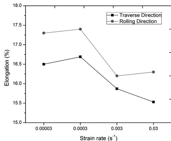
**Figure 4:** Elongation – strain rate relation
