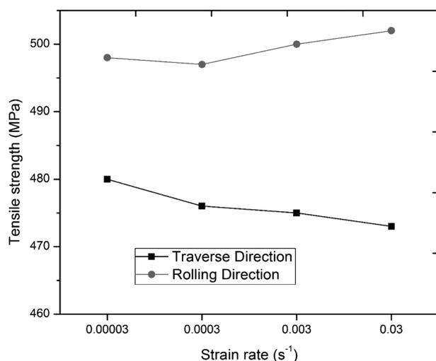
**Figure 3:** Tensile strength – strain rate relation
