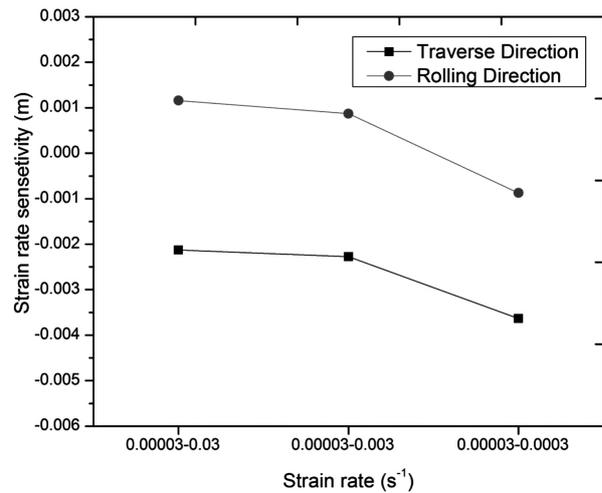
**Figure 7:** Strain rate sensitivity – strain rate relation
