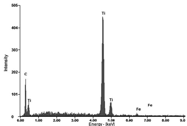
**Figure 4:** Typical EDS spectrum of a TiC particle
