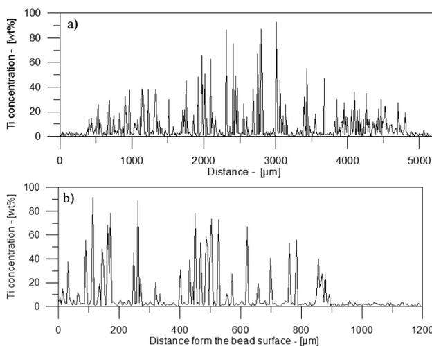
**Figure 2:** EDS line-scan analysis of the cross-section of a SAB produced at a laser power of 1400 W, traverse speed of 0.25 m/min and powder feed rate of 0.0042 g/mm: a) profile taken at the mid-depth of the bead along the line parallel to the bead surface, b) depth profile in the centre of the bead
