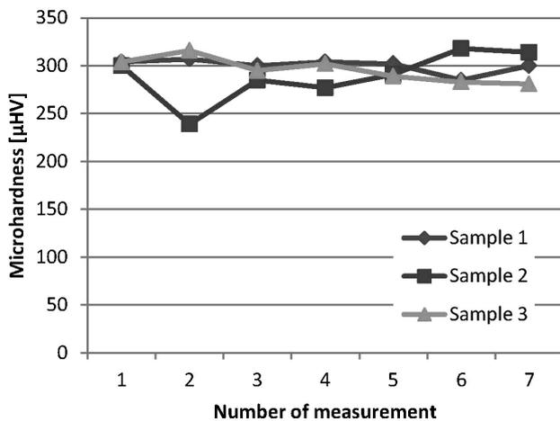
**Figure 8:** Results of the measured microhardness for three samples of Mg<sub>65</sub>Cu<sub>25</sub>Y<sub>10</sub>
