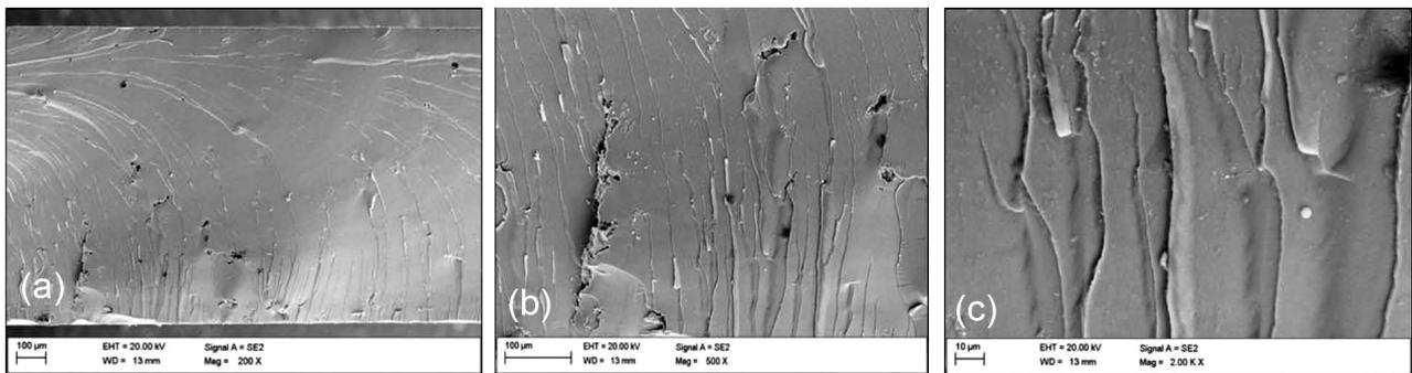
**Figure 5:** Fracture morphology of sample 1 of  $Mg_{65}Cu_{25}Y_{10}$ , SEM images with magnifications of: a) 200×, b) 500×, c) 2000×
