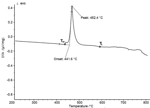
Figure 2: DTA curve for the  $Mg_{65}Cu_{25}Y_{10}$  master alloy
