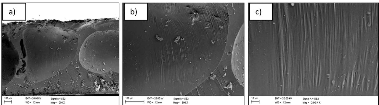
**Figure 7:** Fracture morphology of sample 3 of  $Mg_{65}Cu_{25}Y_{10}$ , SEM images with magnifications of: a) 200×, b) 500×, c) 2000×
