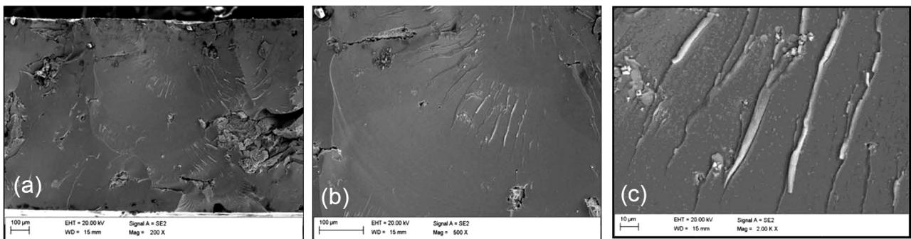
**Figure 6:** Fracture morphology of sample 2 of  $Mg_{65}Cu_{25}Y_{10}$ , SEM images with magnifications of: a) 200×, b) 500×, c) 2000×
