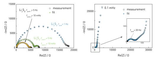
Figure 1: EIS response and fit of symmetrical carbon cells with different polysulfides in the electrolyte (left) and battery cells (right)
