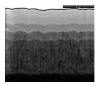
Fig. 1: Functionally graded Ni-W, after heat treatment at 500 °C for 30 min.
