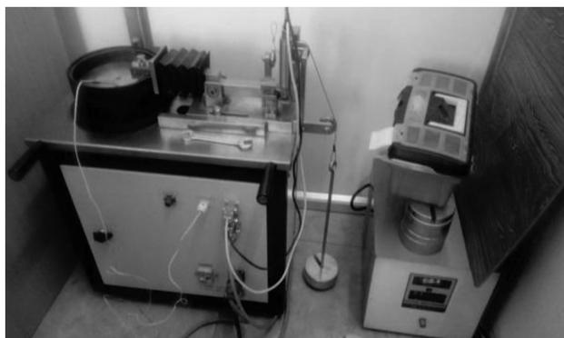
**Figure 3:** Pin-on-disk wear-test apparatus
