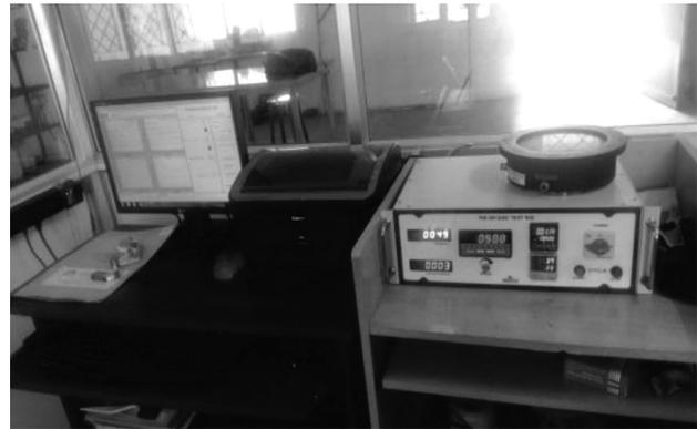
**Figure 4:** Pin-on-disk wear-test apparatus
