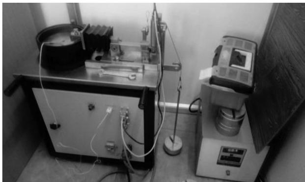
**Figure 3:** Pin-on-disk wear-test apparatus
