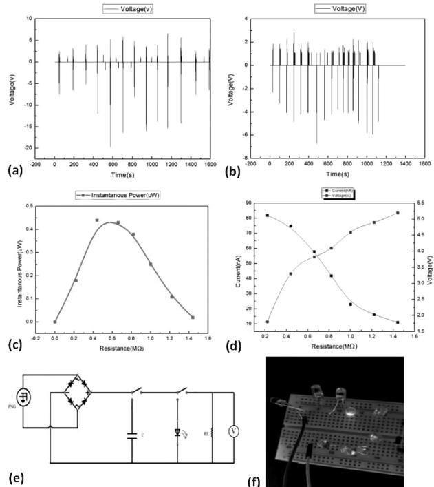
**Figure 4:** a) and b) under different finger pressures rectified output voltage of the PENG, c) fitted curve of the current and voltage output on different external load resistance, d) dependence of the power output on the different external load resistance, e) equivalent bridge rectifier circuit diagram for the DC voltage measurement, capacitor charging and LED lighting performance, f) the LEDs were driven successively by output generated from hand pressing
