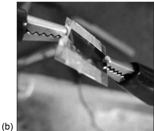
**Figure 1:** a) Schematic diagrams of the PENG fabricating process, b) photograph of the ZnO-PET composite film contact by wires
