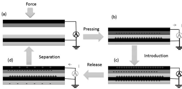
**Figure 3:** Working mechanism of the sandwich-shape PENG. Schematic illustration of the charge-generating process of the PENG. Pushed by the external force from the linear motor, the device will be switching back and forth between the separated state and the contacted state, and there will be an alternating flow of electrons in the external circuit driven by the induced piezoelectric potential. The electric charges move for neutralization after the separation, forming a cycle.
