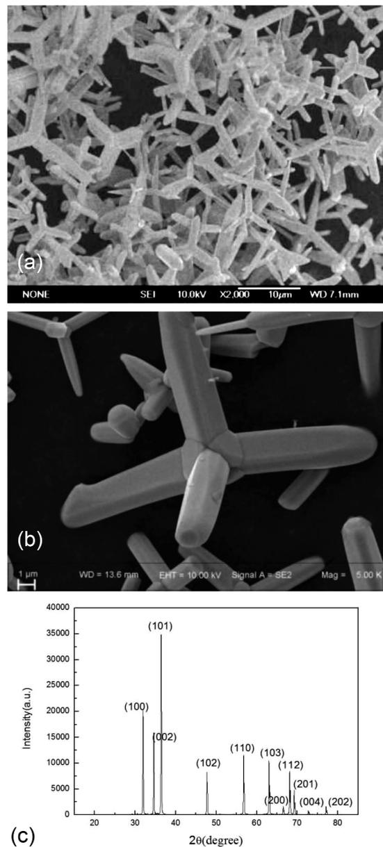
**Figure 2:** Representative SEM images shown up view: a) and b) of ZnO nanotetrapods, c) Rietveld-refinement analysis of XRD spectra of ZnO nanotetrapods
