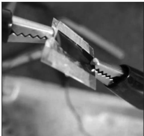
**Figure 1:** a) Schematic diagrams of the PENG fabricating process, b) photograph of the ZnO-PET composite film contact by wires
