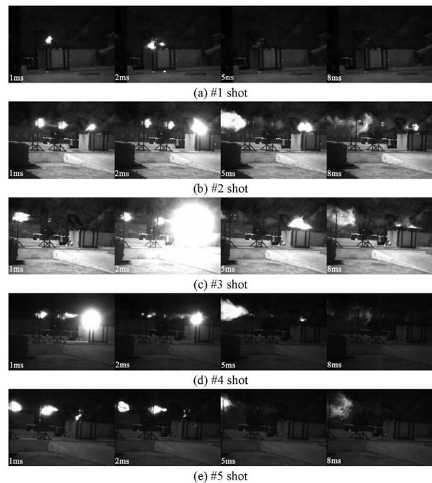
**Figure 4:** Typical high-speed video frames: a) 3-mm-thick plate impacted at  $1450 \text{ m s}^{-1}$ , b) 3-mm-thick plate impacted at  $1560 \text{ m s}^{-1}$ , c) 2-mm-thick plate impacted at  $1348 \text{ m s}^{-1}$ , d) 2-mm-thick plate impacted at  $1218 \text{ m s}^{-1}$ , e) 4.5-mm-thick plate impacted at  $1630 \text{ m s}^{-1}$
