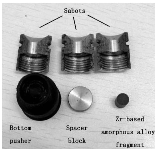
**Figure 1:** Photograph of projectile components
