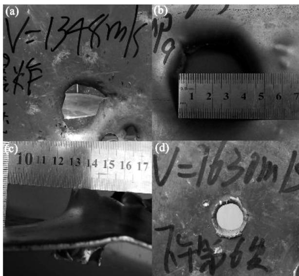
**Figure 3:** Typical photographs of perforated thin plates
