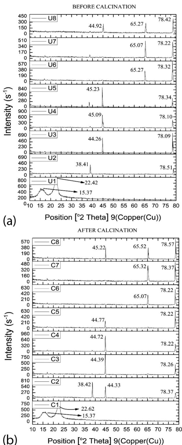
**Figure 2:** XRD diffractograms: a) uncalcinated nanofibres (U1-U8), b) calcinated nanofibres (C1-C8)
