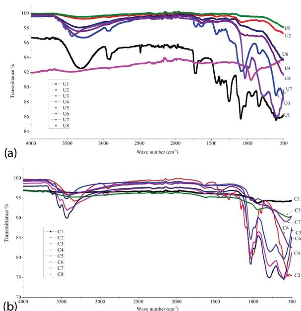
**Figure 3:** FTIR spectrum of: a) uncalcinated nanofibres, b) calcinated nanofibres
