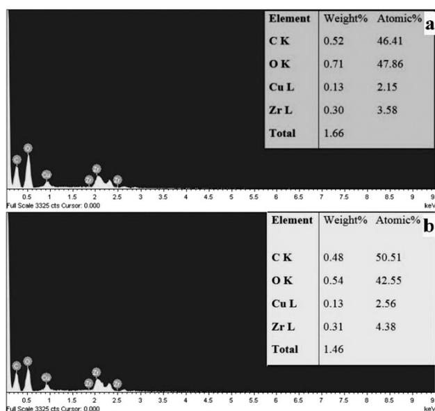
Figure 8: EDX spectrum of: a) U3 Sample, b) C3 Sample
