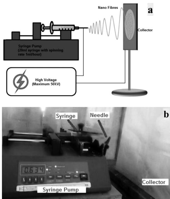
**Figure 1:** Electrospinning apparatus: a) schematic view and b) photograph
