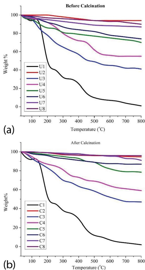
**Figure 4:** TGA curves of: a) uncalcinated nanofibres, b) calcinated nanofibres
