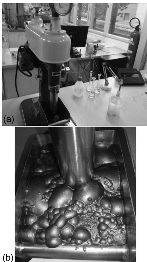
**Figure 3:** Denver flotation cell in operation (on the left) and sample flotation process with good adherence of carbon in the bubble-froth (on the right)
