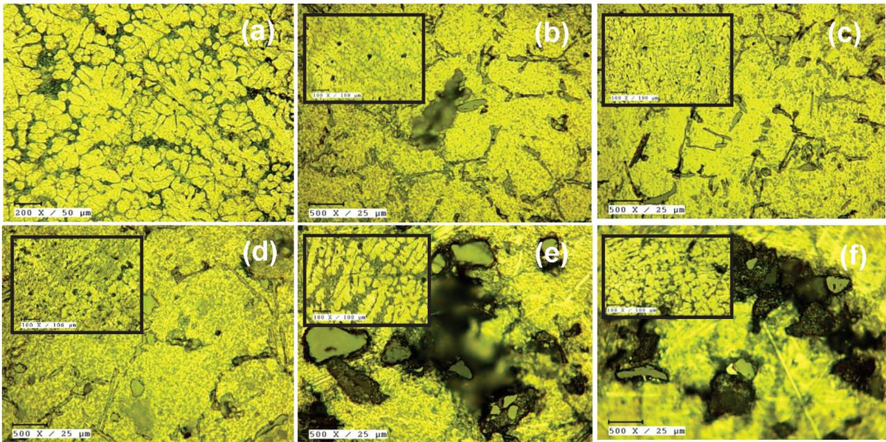
**Figure 1:** Optical microstructures of the stir-cast alloy and composites a) LM25 alloy, b) composite A, c) composite B, d) composite C, e) composite D, and f) composite E at 500 × mag./25 μm (the insert graph at a magnification of 100 ×/100 μm)
