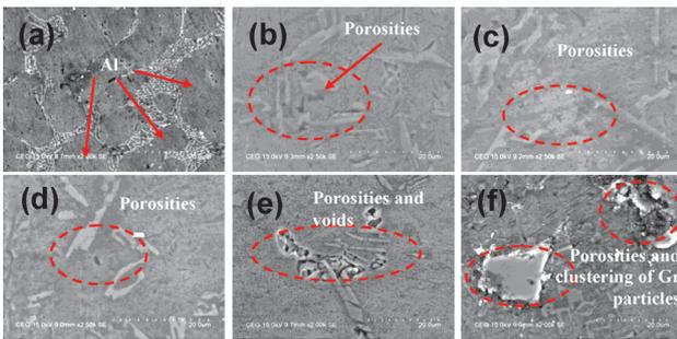
**Figure 2:** SEM images of the LM25 alloy and composites: a) LM25 alloy, b) composite B, c) composite B, d) composite C, e) composite D, and f) composite E
