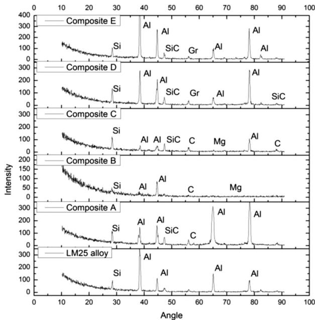
**Figure 3:** XRD patterns of the LM25 alloy and composites: a) LM25 alloy, b) composite A, c) composite B, d) composite C, e) composite D, and f) composite E
