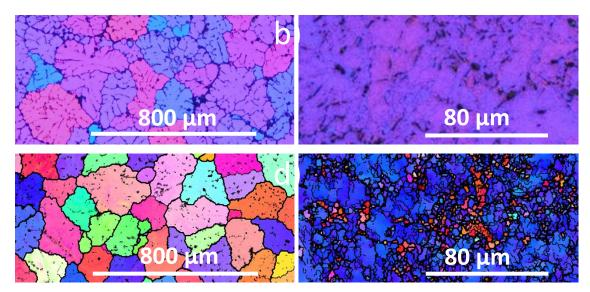
Figure 1: Microstructure of alloy 2011 with 0.17 wt% Si: a) optical micrograph of cast disc, c) optical micrograph of extruded and artificially aged rod, c) IPFZ map of cast disc, d) IPFZ map of extruded and artificially aged rod.
