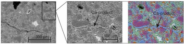
Figure 1: Crack in cement paste filled with secondary Ca-products ("Ca halo") as a consequence of the ACR.
