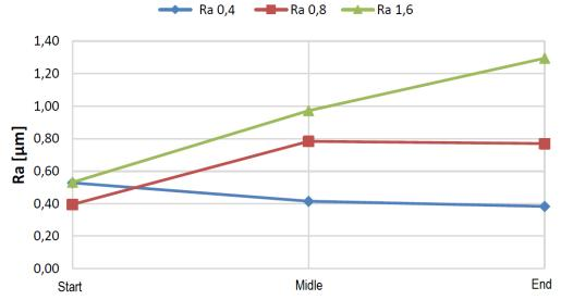
The visualization of roughness in points with varying distance from the gate
