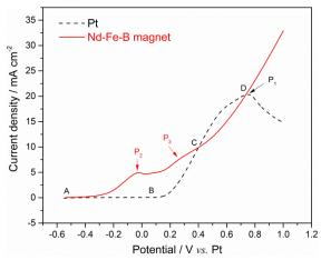
**Fig. 1** Linear sweep voltammetry of a Pt wire working electrode (black dashed curve) and the initial Nd–Fe–B magnet scrap (red solid curve) in DMF containing 0.3 mol  $L^{-1}$  FeCl<sub>2</sub>, 40 mV s<sup>-1</sup>, room temperature.
