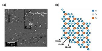
Figure 1: (a) SEM micrograph combined with EDS of the sample Al<sub>52</sub>Cr<sub>14</sub>Sc<sub>34</sub> (b) The crystal structure model of the ternary Laves phase in [0 0 0 1] zone axes.
