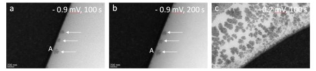
Figure 1: (a,b) BF TEM micrographs of Ni deposits at applied potential of -0.9 mV after 100 s and 200 s at low electron beam dose. Ni deposits are clearly observed at the electrode/liquid interface. (c) Nucleation of Ni nanoparticles from the solution due to radiolysis of the water at high dose of electron beam.
