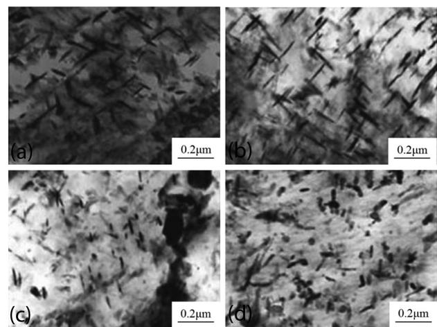
**Figure 9:** TEM micrographs of 34CrNiMo6 specimens quenched in oil (870 °C/30 min) and tempered at different tempering temperatures: a) as quenched in oil (870 °C/30 min), b) quenched and tempered at 630 °C for 3 h, c) quenched and tempered at 660 °C for 3 h, d) quenched and tempered at 690 °C for 3 h
