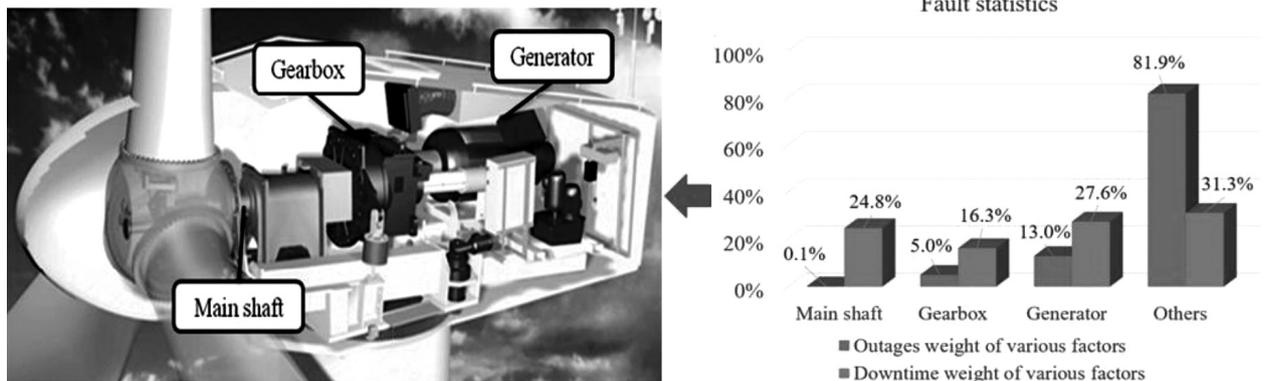
**Figure 1:** Outage and downtime weights of wind-turbine faults
