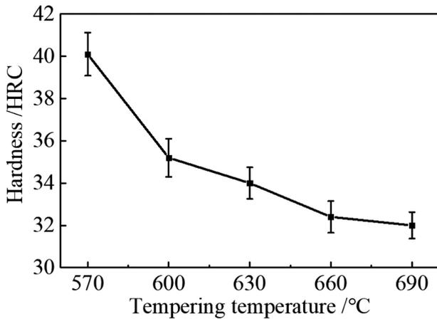
Figure 5: Evolutions of hardness with the tempering temperature
