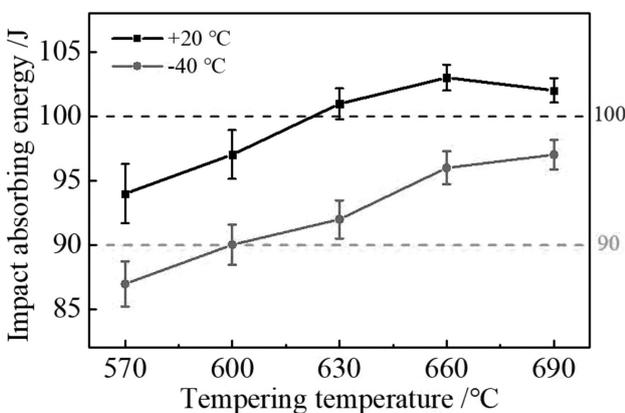
Figure 6: Evolutions of impact-absorbing energy with the tempering temperature under different temperatures
