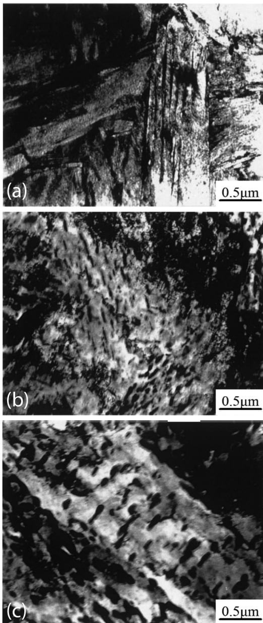
**Figure 8:** TEM micrographs of 34CrNiMo6 specimens quenched in oil (870 °C/30 min) and tempered at different tempering temperatures: a) as quenched in oil (870 °C/30 min), b) quenched and tempered at 570 °C, c) quenched and tempered at 660 °C
