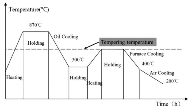
Figure 3: Flow chart of the main-shaft heat treatment
