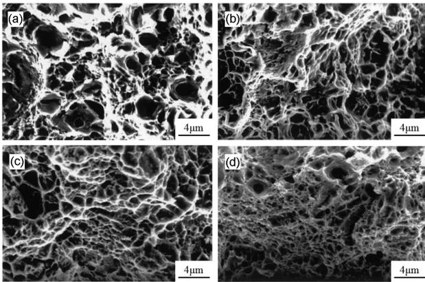
**Figure 10:** Fracture morphologies of specimens quenched in oil (870 °C/30 min) and tempered at different tempering temperatures: a) as quenched in oil (870 °C/30 min), b) quenched and tempered at 570 °C for 3 h, c) quenched and tempered at 630 °C for 3 h, d) quenched and tempered at 660 °C for 3 h
