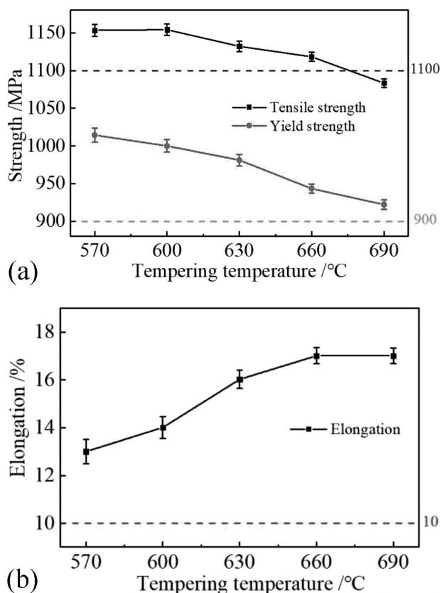
**Figure 4:** Evolutions of strength and elongation with the tempering temperature: a) tensile strength and yield strength, b) elongation after breakage
