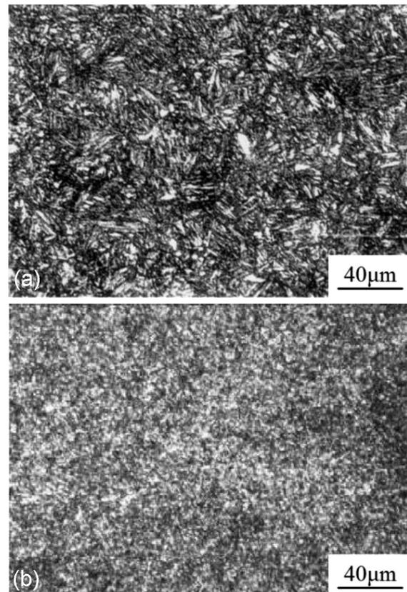
Figure 7: Metallographs of 34CrNiMo6 specimens quenched in oil (870 °C/30 min) and then tempered at 660 °C: a) quenched in oil (870 °C/30 min), b) quenched and tempered at 660 °C
