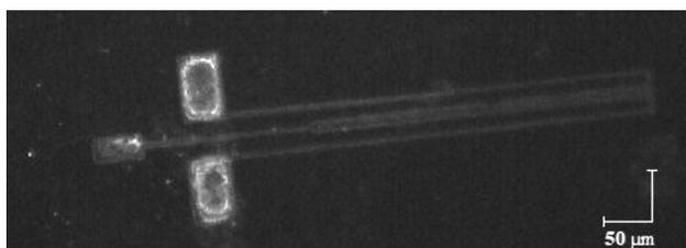
**Figure 9:** Image of the actuator fabricated with the P $\mu$ SL method (the NanoArch™ device's camera)
