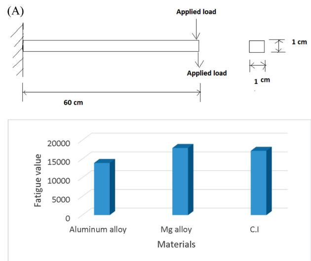
**Figure 6:** Fatigue analysis: a) CAD-model for fatigue load condition, b) fatigue value for Mg, Al and cast iron
