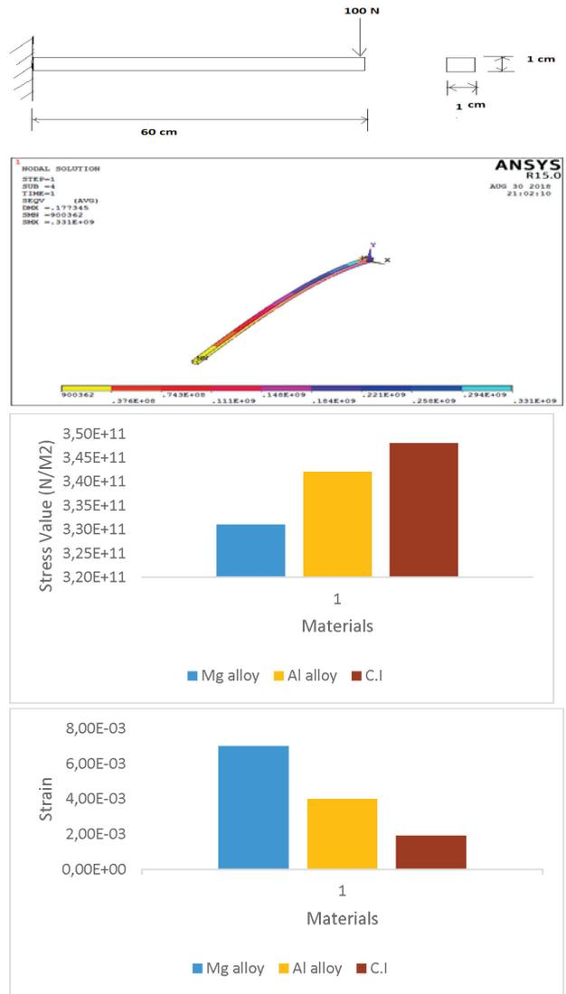
**Figure 3:** Nonlinear static analysis: a) CAD model for static load condition, b) stress analysis of Mg, c) stress curve, d) strain curve
