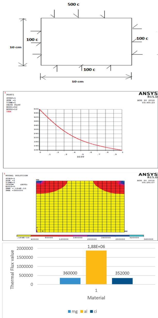
**Figure 4:** Thermal analysis: a) CAD-model for thermal load condition, b) temperature distribution curve (node number vs. temperature) for Mg alloy, c) thermal flux analysis of Mg alloy, d) thermal flux curve for all the three materials
