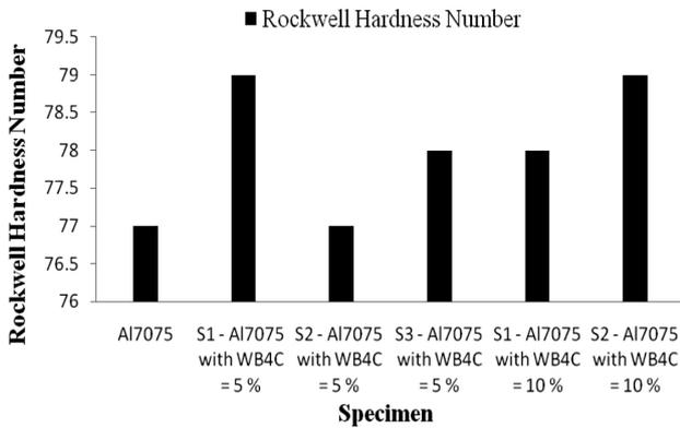
Figure 8: Rockwell hardness numbers from the experiments
