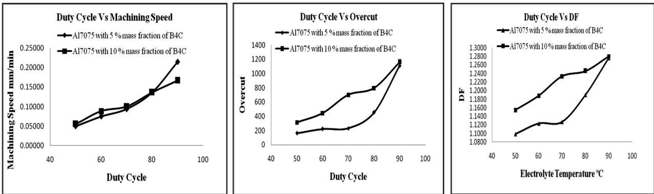
Figure 5: a) Effect of duty cycle on the machining speed, b) effect of duty cycle on the overcut, c) effect of duty cycle on the DF
