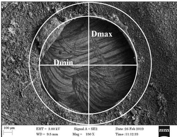
**Figure 1:** Delamination factor
