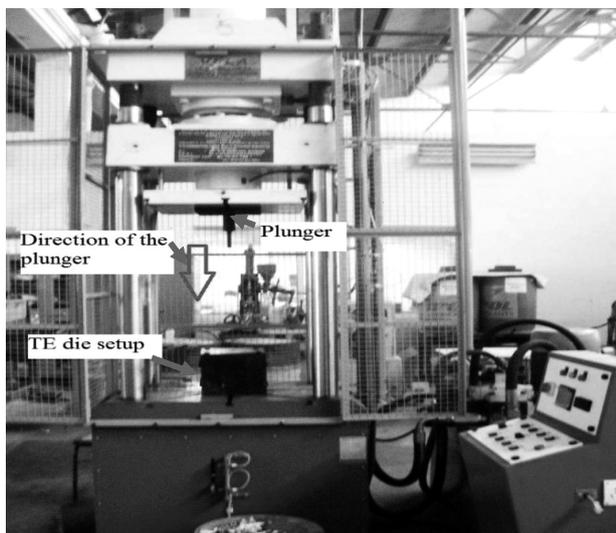
**Figure 1:** Four-column vertical hydraulic press for the TE forming process
