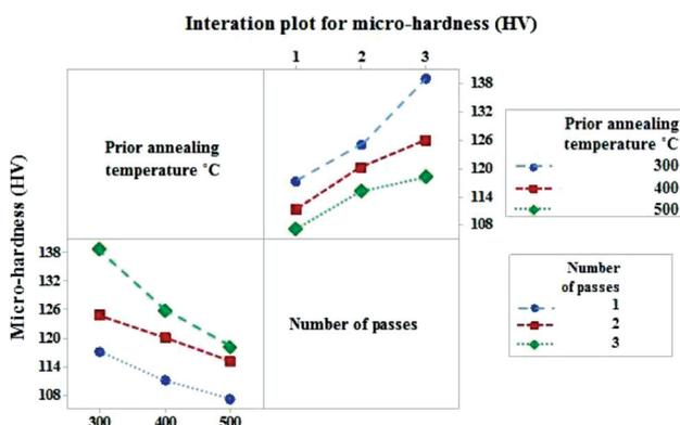
**Figure 6:** Micro-hardness values for the AA 7075 aluminum alloy corresponding to different treatments
