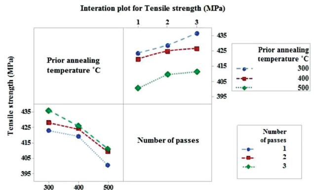
**Figure 4:** Tensile-strength values corresponding to different treatments
