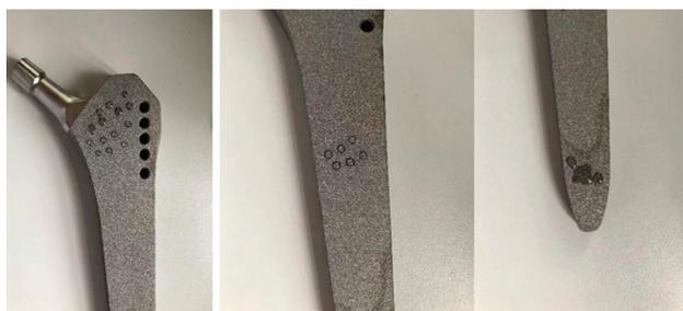
Figure 4: Static water contact-angle measuring site on new stem
