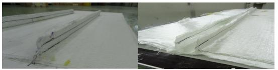
Fig.1 Composite composition before vacuum infusion technology
