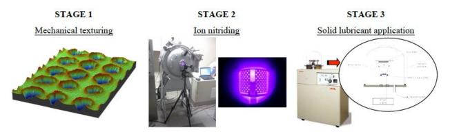
Fig.1. Multiplex surface treatment applied for Ti6Al4V
