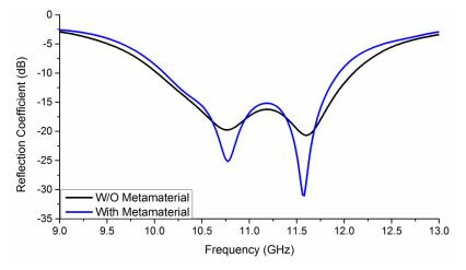
Fig. 1. Reflection coefficient of proposed antenna.
