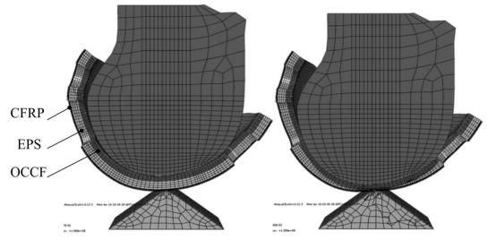
Fig. 1. Numerical simulation of helmet test according to ČSN EN 1078 (before and during impact).
