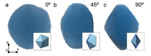
Figure 1: 3D visualizations of the reconstruction showing the atomic lattice of a Au nanodecahedron.
