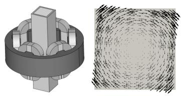
Figure 1: A sample geometry of the M-EMS (left) and the time averaged force on the horizontal plane in the mould (right).
