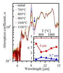
Fig.1 Relationship between attainment temperature and absorption coefficient
