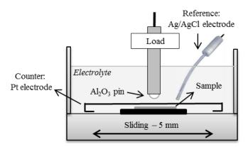
Figure: Set-up of tribocorrosion experiment
