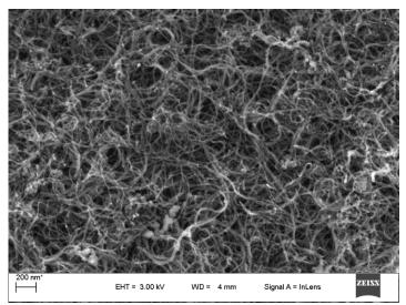
Fig.1. SEM images of carbon nanotubes surface topography
