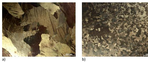
Figure 1. Microstructure of the AIMg5 aluminium alloy subjected to the a) 2 ECAP pass route Bc, b) 2 ECAP pass route Bc and annealed at 350 °C for 30 min
