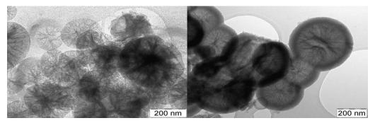
Figure 1: TEM pictures of pristine (left) and surface modified (right) silica particles.
