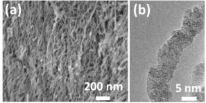
Fig. 1 (a) SEM image and (b) TEM image of  $SiO_2/SnO_2$  nanofibers
