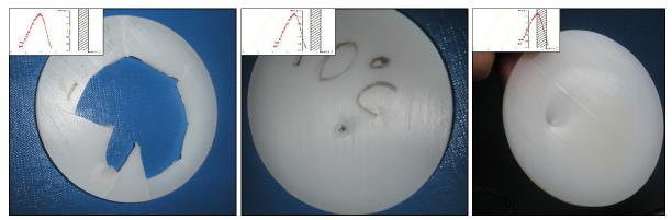
Figure 1: High-rate impact characterization, examples of PA6 impact behavior at different temperatures
