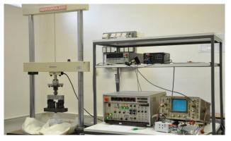
Figure 1 Set up for measuring of fatigue properties
