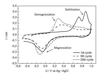
Figure 1: Cyclic voltammogram of  $LiMn_2O_4$  in 0,1 M Mg(NO<sub>3</sub>)<sub>2(aq)</sub> in potential window between -0.5 and 1.0 V vs Ag / AgCl at sweep rate 5 mV s<sup>-1</sup>. Peaks indicating magnesium intercalation are visible.
