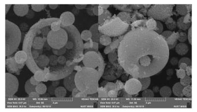
Figure 1 – Images captured with the scanning electron microscope Tescan Vega 3, nanostructured  $Mn_2O_3$  microspheres aged at high temperatures, obtained by ultrasonic spray pyrolysis.
