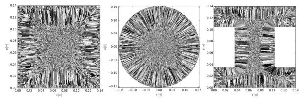
Figure 1: Final microstructure in the CC of steel for different cross sections of billet.
