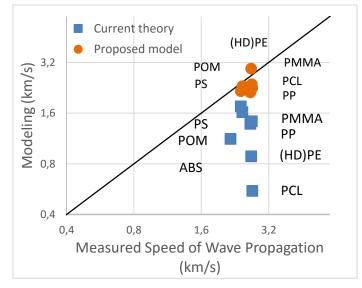
Figure 1: Comparison between current wave propagation theory (blue square markers) and proposed wave propagation model (orange circle markers). Results closer to the diagonal line are better.
